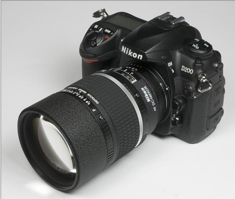
The build quality of the lens is excellent thanks to combination of metal and plastic parts with a Nikon "pro style" crinkle finish. The length of the lens remains constant regardless of the focus setting and the front element does not rotate due to an RF (Rear Focusing) design. A nice and almost forgotten approach is the build-in lens hood (telescope style). I would really wish that this old "fashion" will see a revival again.
