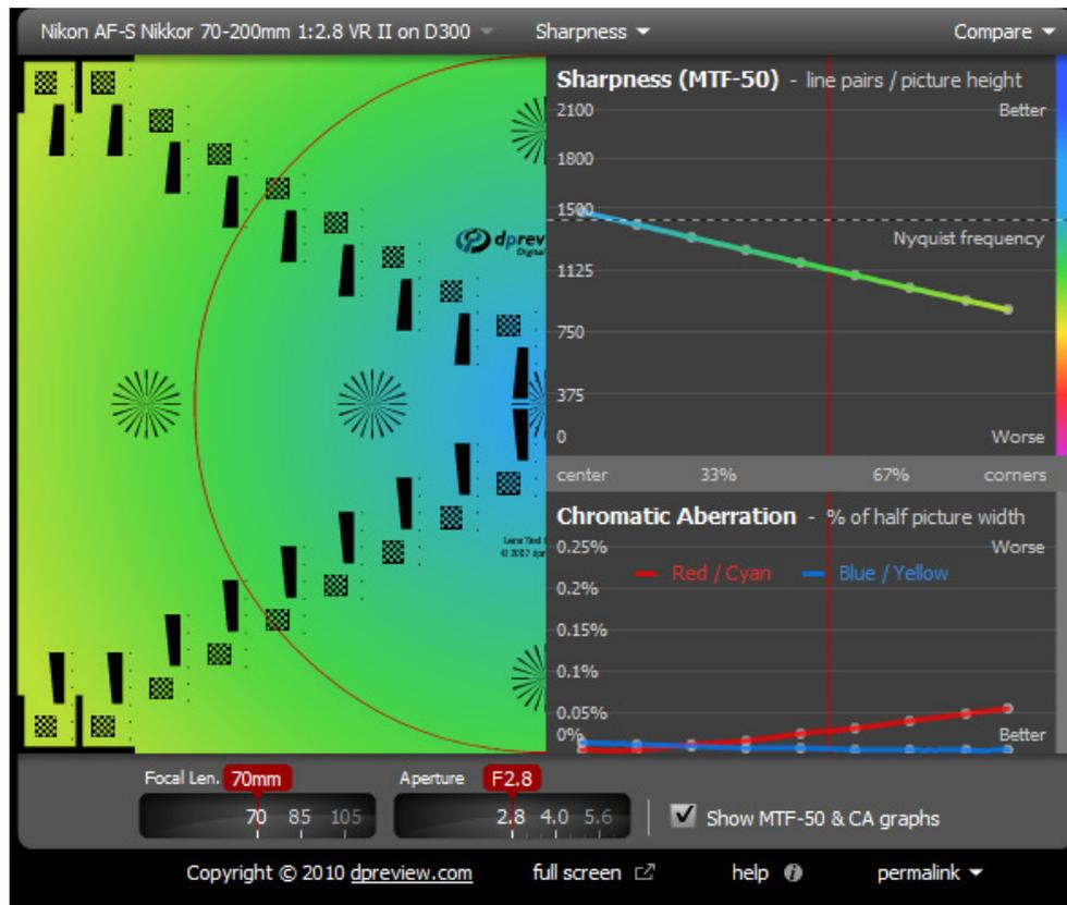
NOTE the line marked 'Nyquist Frequency' indicates the maximum theoretical resolution of the camera body used for testing. Whenever the measured numbers exceed this value, this simply indicates that the lens out-resolves the sensor at this point - the calculated MTF values themselves become meaningless.
