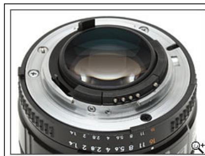
The lens uses Nikon's venerable F mount, and will fit all of their DSLRs, both DX and FX format. It communicates with the body electronically via an array of contact pins, with mechanical control of the aperture using a metal lever.
